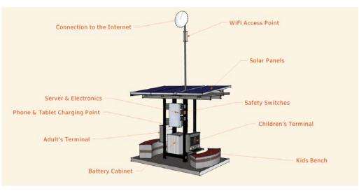
One long side contains access to the HELLO HUB systems and control components, and the other long side contains an electronic workbench and charging shelf.
